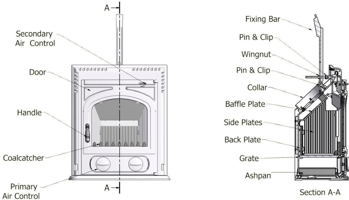
Fig 2 – FW5i Stove Assembly and controls
