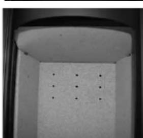
Fit Lower baffle brick and support with 2 x steel pins in lower holes in side brick.
