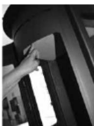
Place Top baffle in position against L shaped lugs leaving 5cm gap at rear of stove.
