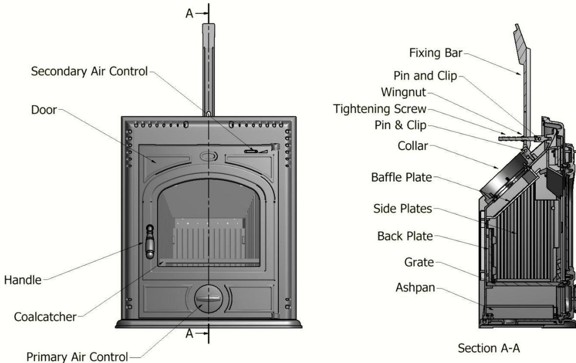
Fig 2 – SR5i Stove Assembly and controls
