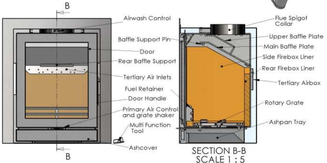
Fig 2 – TR5c, TR8c Stove Assembly and controls
