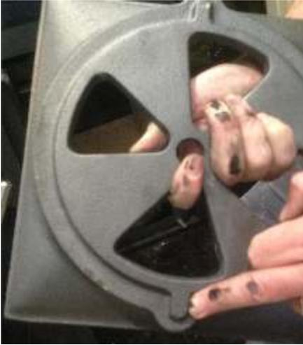
When re- installing base grate make sure lugs under the grate are in the quarter to three position and match the cutout in the base of the stove.
