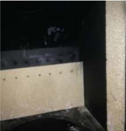
Remove side rear right brick , Remove side left brick
