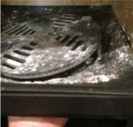
Remove riddling grate, Place hand through ashpan and lift the cast iron riddling grate up and remove.
