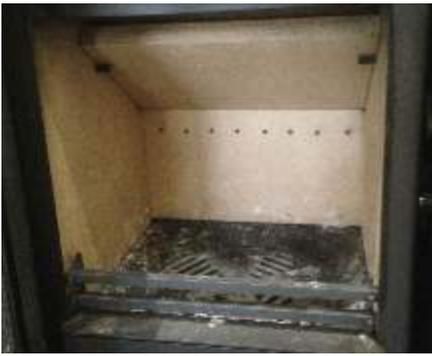
To remove a vermiculite brick set take the following steps.
