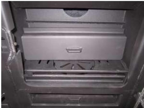
Fig 10 - Insert baffle with chamfers down
