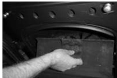
**Grasp and lift the baffle off the ledge at the rear of the combustion chamber, turning the baffle as you remove it through the door.**
